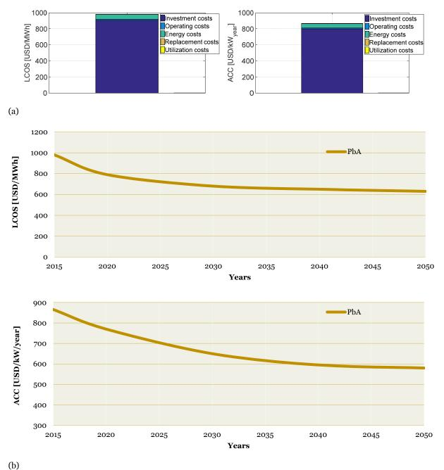
Fig. 31.) LCOS & ACC of the Pb-A magazine broken down into costs, b) change of LCOS & ACC in the 2015-2050 perspective.
