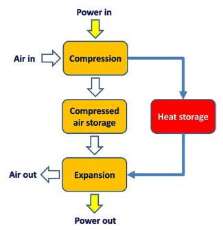
Fig. 9. A-CAES power plant operation principle – own study
