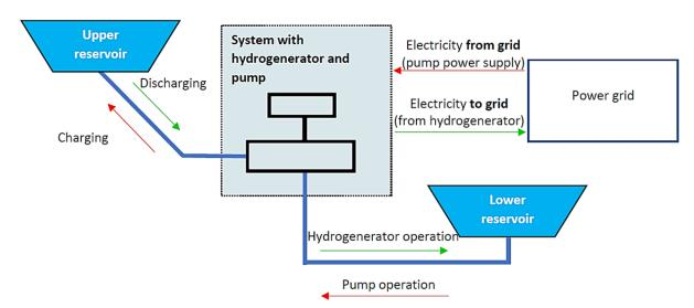
Fig. 3. Principle of operation of a pumped storage power plant - own study
