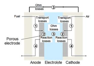
**Fig. 20.** A simplified diagram of the fuel cell, together with an indication of the location of characteristic losses occurring during its operation<sup>142</sup>
