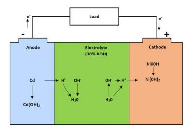
Fig. 28. Functional diagram of the Ni-Cd battery during discharge - own study
