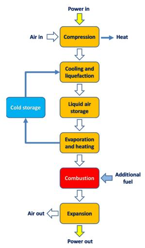
Fig. 13. Principle of d-LAES power plant operation – own study
