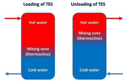
Fig. 41. Principle of operation of the TES magazine – own study.
