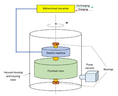
Fig. 16. The principle of kinetic inertia – own study
