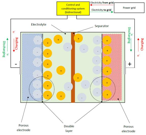
Fig. 38. Double layer supercapacitor diagram (UC / EDLC) - own study
