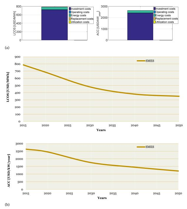
Fig. 37.a) LCOS & ACC of the SMES storage broken down into costs, b) change of LCOS & ACC in the 2015-2050 perspective
