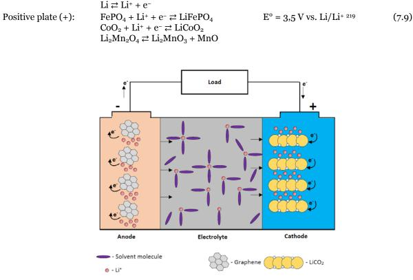
Fig. 30. Diagram of operation of lithium battery works - own study
