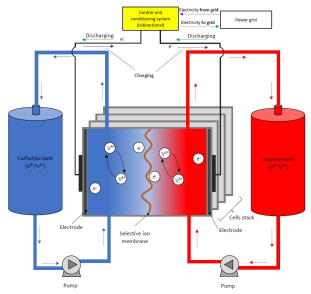
Fig. 34. VRFB flow-through battery operation diagram - own study
