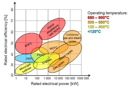
**Fig. 21.** Graphic presentation of the range of applicability of selected power systems, including rated electrical power, efficiency and operating temperature<sup>147</sup>
