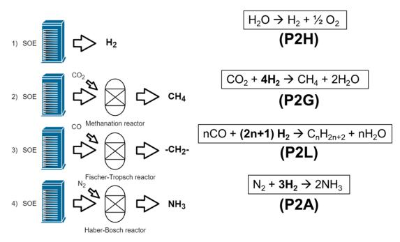
Fig. 26. A list of the four most important technologies under the common name of P2X
