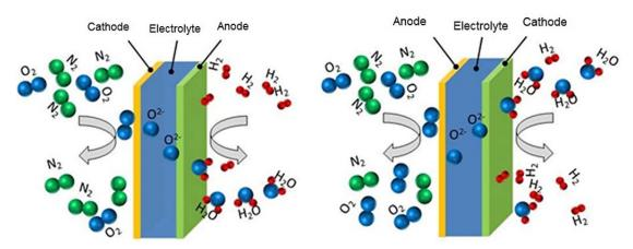
**Fig. 18.**SOC cell operating in SOE electrolyser mode (left) and in SOFC fuel cell mode (right). Based on
