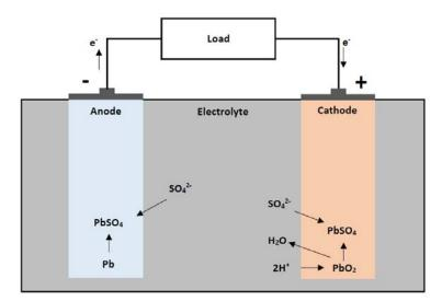
Fig. 27. Functional diagram of the Pb-A battery during discharge - own study
