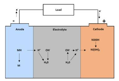
Fig. 29. Diagram of NiMH battery operation during the discharge process - own study
