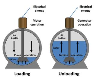
**Fig. 4.** Principle of operation and simplified construction scheme of the bottom tank of a pumped storage power plant in the StEnSea technology – own study, based on <sup>76</sup>.
