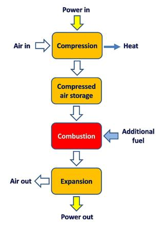
Fig. 10. Principle of d-CAES power plant operation – own study
