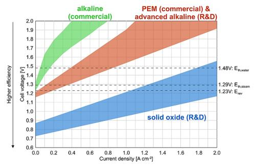
Fig. 22.Comparison of parameters: alkaline, PEM and solid oxide electrolysers. Based on<sup>151</sup>, supplemented with unpublished data from Institute of Power Engineering
