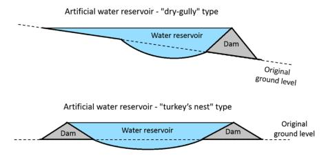
Fig. 7. Types of potential locations of pumped storage power plant reservoirs - own study
