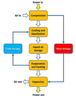
Fig. 12. A-LAES power plant operation principle - own study
